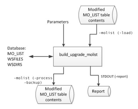
The following diagram illustrates the data input and output flow:
