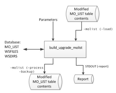
The following diagram illustrates the data input and output flow:
