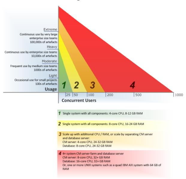
Use the chart above to determine appropriate hardware needs for different usage zones, based on the expected number of active concurrent users. These recommendations are based on Serena internal performance testing.
