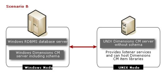
The locally installed Dimensions CM server is like an Agent installation (see "Dimensions CM Agent Components" on page 70) in that it will provide Dimensions CM listener services and the dmcli command client, but the Common Tools (Dimensions web client, Administration Console, and Common Tomcat server) will also be installed.
