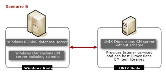
For this, the remote database server requires both the RDBMS and Dimensions CM binaries to be installed and for a Dimensions CM schema to have been created in that RDBMS. To enable network connections between the nodes, the remote database server must be running an additional process. For Oracle, this is the case if the TNS Listener has been started up.
