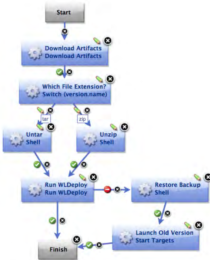
Figure 2. Process Editor with a Component Process Containing a Switch Step
